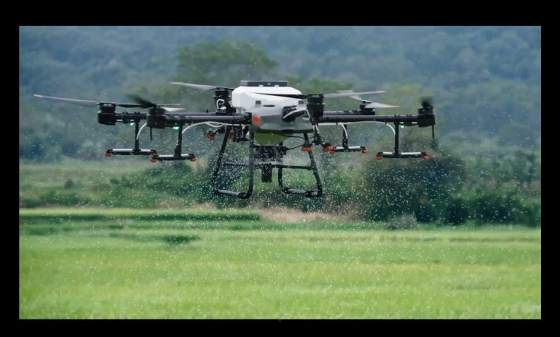
With revolutionary branch-targeting technology and adjustable arms, the Agras T30 penetrates thick canopies with oblique spraying, ensuring an even application of liquid pesticides and doubling the number of droplets.
