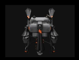
The Agras T30 can be folded by 80%, making it easier to transport. This folding mechanism uses quick-snap locking, redundancies, and an in-app alert to help ensure safe operation.
